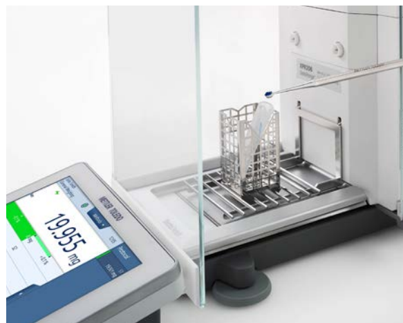
Figure 7: Weighing with an ErgoClip, a small metal basket, which acts as a tare vessel holder and shields the vessel from electrostatic charges.
